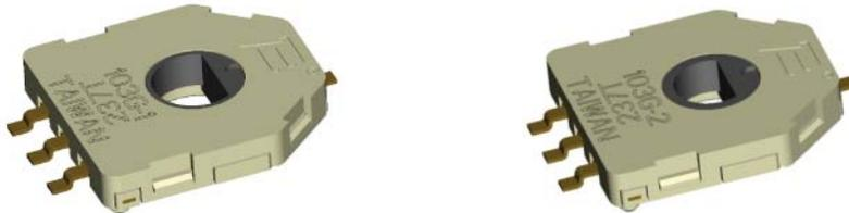
And last but not least, we have increased the number of available resistance values from one to six; ranging from 2.5K ohms to 100K ohms. These additional resistances give engineers the freedom and flexibility to design various components into their circuits without limiting their choices to 10K ohms, which is the only value currently available in the marketplace.
