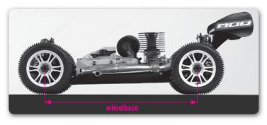
Wheelbase refers to the horizontal distance between the front and rear axles. Changes to wheelbase can have a dramatic effect on the handling of your car, since it readjusts the distribution of weight on the wheels, which adjusts traction. Not all RC cars have the option to adjust the wheelbase.
