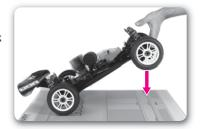
• Using the droop gauge, measure the ride height value at the front of the car.
