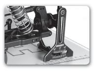
Each graduated mark indicates a 1° camber value. You should be able to set camber with a resolution of  $0.5^{\circ}$ .
