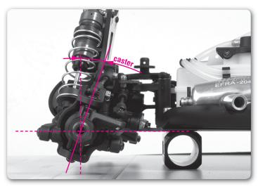
Caster describes the angle of the front steering block with respect to a line perpendicular to the ground. The primary purpose of having caster is to have a self-centering steering system. Caster angle affects on- and off-power steering, as it tilts the chassis more or less depending on how much caster is applied.
