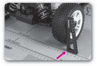
• Make sure the rear wheels rest on the rear track-width graduation marks.
