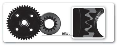
Proper gear mesh between the center diff spur gear and the clutchbell pinion gear is vitally important to obtain optimal drivetrain operation, smoothness, and efficiency. Improper gear mesh can result in a binding drivetrain, overstressed clutch/diff components, and chipped or broken gear teeth.
