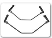
The front anti-roll bar affects mainly off-power steering at corner entry.
