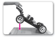
• Using the droop gauge, measure the ride height value at the rear of the car.
