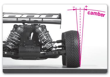
Camber is the angle of a wheel to the surface on which the car is resting (with wheels and shock absorbers mounted).
