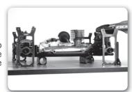
• Push on the car so the chassis rests flat atop both droop blocks at front and rear.
