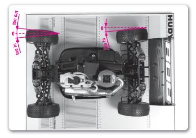
Toe is the angle of the wheels when looked at from above the car. Toe is used to stabilize the car at the expense of traction, as it introduces friction and therefore some slip in the tires.
