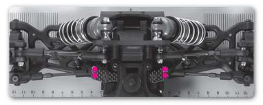
Adjust the Ackermann angle by moving the inside ends of the steering rods into different holes in the steering plate.
