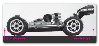
Ride height is the height of the chassis in relation to the surface it is sitting on, with the car ready to run. Ride height affects the car's traction since it alters the car's center of gravity and roll center. Differences in ride height alter the car's attitude (angle of the chassis) which in an off-road vehicle can effect how it jumps and lands. Because of changes in suspension geometry and ground clearance, there are negative consequences to altering ride height too much.
