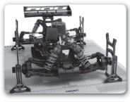
• Read the caster angle from the side of the front set-up stands.
