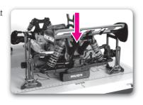
Read the camber setting from the camber gauge of each of the four set-up stands.
