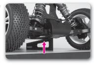
• Lift the rear of the car and let it fall back to the set-up board by itself.
