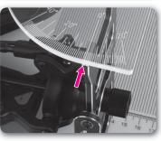
gauge. Each graduated mark indicates a 1° toe value. You should be able to set toe with a resolution of 0.5°.
