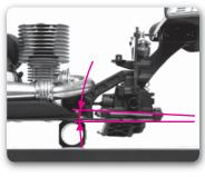
start of a race. In order to prevent 100% of the car's weight transfer force from being exerted onto the soft rear springs, anti-squat is used to allow a certain percentage of the weight transfer to be absorbed by the rear lower arm motion.
