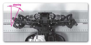
Steering systems may be adjustable for Ackermann angle, servo saver preload, and bump steer.
