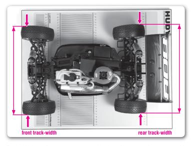
Track-width is the distance between the outside edges of the wheels, front or rear, and it affects the car's handling and steering response. It is important that front or rear track-width is adjusted symmetrically, meaning that the left and right wheels (at one end of the car) must be the same distance from the centerline of the chassis.
