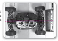
• Make sure the front wheels rest on the front track-width graduation marks. The amount of toe-in/toe-out has direct influence on the track width so make sure to measure at the part where the car is widest.
